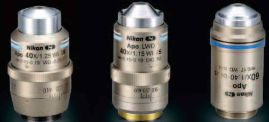
CFI Apochromat 40x WI S, NA 1.25, WD 0.18 CFI Apochromat LWD 40x WI S, NA 1.15, WD 0.60 CFI Apochromat 60x oil S, NA 1.40, WD 0.14
