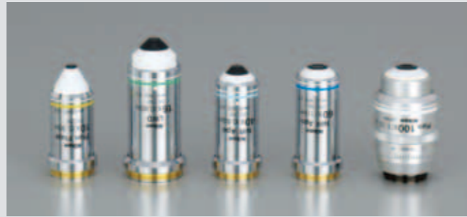
CFI Plan Fluor 10x W, NA 0.3, W.D. 3.5mm CFI75 LWD 16x W, NA 0.8, W.D. 3.0mm CFI Apochromat 40x W NIR, NA 0.8, W.D. 3.5mm CFI Apochromat 60x W NIR, NA 1.0, W.D. 2.8mm CFI Plan 100x W, NA 1.1, W.D. 2.5mm
