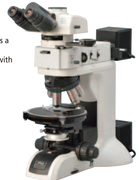
ECLIPSE LV100N POL (Diascopic/Episcopic illumination type)
